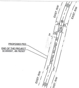
PROPOSED COMCAST UNDERGROUND DIRECTIONAL BORE 4' MINIMUM DEPTH AT ALL POINTS 1 24CT FIBER CABLE NO OTHER BURIED UTILITIES EXIST
